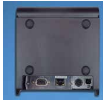
Triple Interface Standard – Serial+Ethernet+USB – Cash Drawer Port Standard
