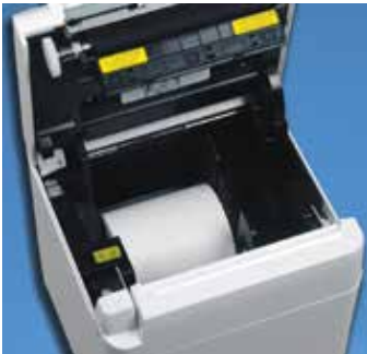
Drop and Print Paper Loading With Standard Paper Width Selector
