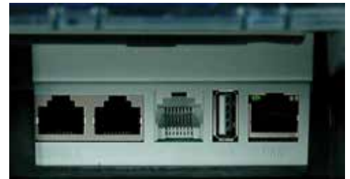
3 RS232C, 1 USB, 1 Ethernet Ports Hidden Behind a Convenient, Easy to Access Door
